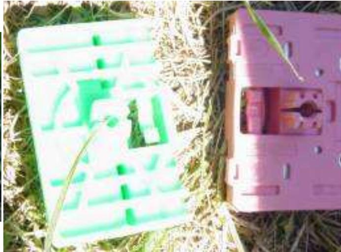
Sometimes, a good blob of araldite to hold the cable nipple in place works fine, but mine didn't hold. My clips were green, and the plastic is quite slippery. It's also brittle: when I tried to remove one to get a good photo, it broke. Maybe the blue ones stick better? If you want to try the araldite, do that, let it set for a bit, and then join us below after we replace the regulator mechanism.
