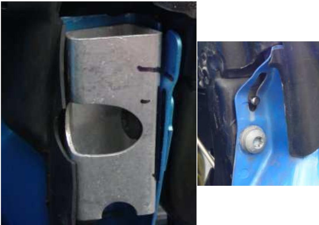
Undo the bolts and remove the bracket. The subframe will drop a little, but won't fall out. Disconnect the cable from the window motor, and unclip from the cable clips on the subframe. Pull off the trim from behind the mirror, pull out the foam, and disconnect and unclip the cable here too.
