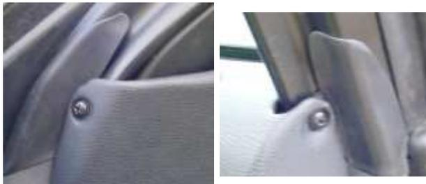
Remove the screw under the door pull (circled, but not clear in my photo), pull out the cover, and remove the 2 screws underneath. The door card will now lift upwards and off. Be careful of the cables.
