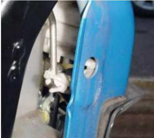
Reconnect the window motor cable and mirror cable (replace the foam here too), and secure with cable ties to the subframe. HINT: At this point, you might want to get the window switch out of the door card, connect it, and test the window!
