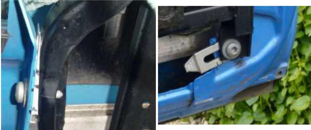
Now mark the position of the bracket (front top of the door) and the bolt and dowel (back top of door). I drew around the bolt with the marker pen. Note that at the front, the dowel fits into the bracket.
