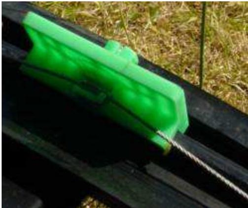
Replace the clips with the new ones, then grease all the runners and cables, and carry on down the page to 'Refitting'.
